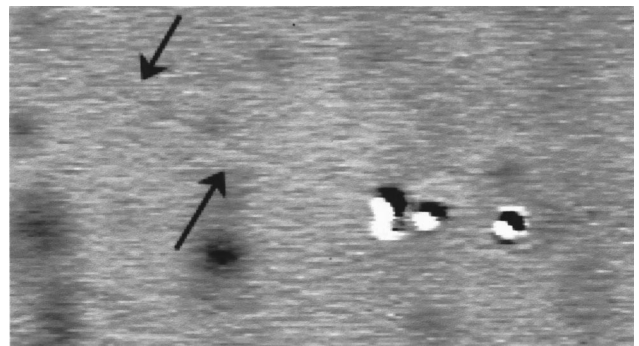
FIG. 3. Differential interface contrast (DIC) image showing a microtubule (indicated by the arrows) to which three 0.3 \mu m beads were attached. Single beam optical tweezers were used in order to buckle the microtubule by applying force on the right-most bead that was attached to the filament. DIC optics based on \times 100/1.3 NA objective (Zeiss), allows the simultaneous observation of the beads and the microtubules. The optical tweezers are based on an 830 nm single-mode laser diode with a maximum power of 200 mW (SDL-5432-H1, SDL Inc., San Jose, CA). The horizontal dimension of the figure is 20 \mu m .
